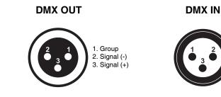
1. Group 2. Signal (-) 3. Signal (+) If you are using controllers with this occupation, you can connect the DMX-output of the controller directly with the DMX-input of the first fixture in the DMX-chain. If you wish to connect DMX-controllers with other XLR-outputs, you need to use adapter-cables.
