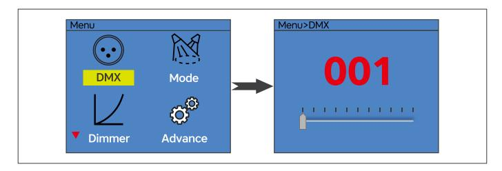
If you set a different address, each unit will start to listen to the channel number you have set, based on the quantity of control channels of the unit. That means changing the settings of one channel will affect only the selected fixture.
