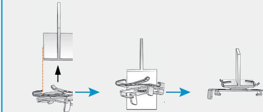
**2** Adjust the Mounting Kit's direction, put the track vertically into the Mounting Kit, rotate left and fix (as picture shows)
