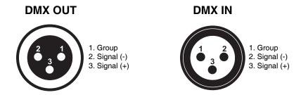
If you are using controllers with this occupation, you can connect the DMX-output of the controller directly with the DMX-input of the first fixture in the DMX-chain. If you wish to connect DMX-controllers with other XLR-outputs, you need to use adapter-cables.
